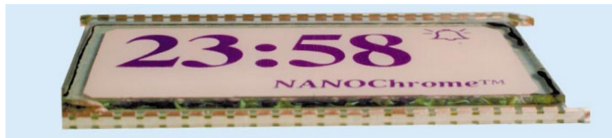
Figure 2 Prototype of a fast switching, high-contrast electrochromic device viewed at a low angle.
